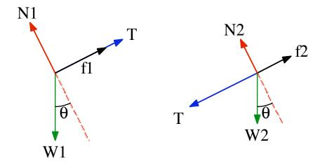
Since the masses move along the ramp, there is no motion in the direction perpendicular to the ramp. The net force in this direction must thus be equal to 0. For block 1 we thus require that
