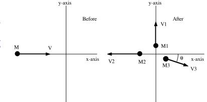
$$(m_3 v_3)^2 = (MV + m_2 v_2)^2 + (m_1 v_1)^2$$
