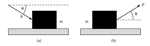
Instead of pushing the block with a force P, we can pull the block with the same force P (see Figure b).
