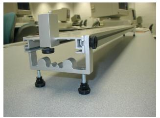
Dynamics Track is level and the cart does not roll one way or the other.
