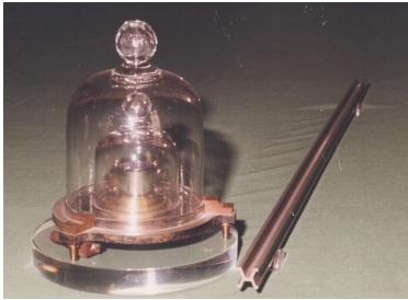
The old standard of the kg and the old standard of the m.
