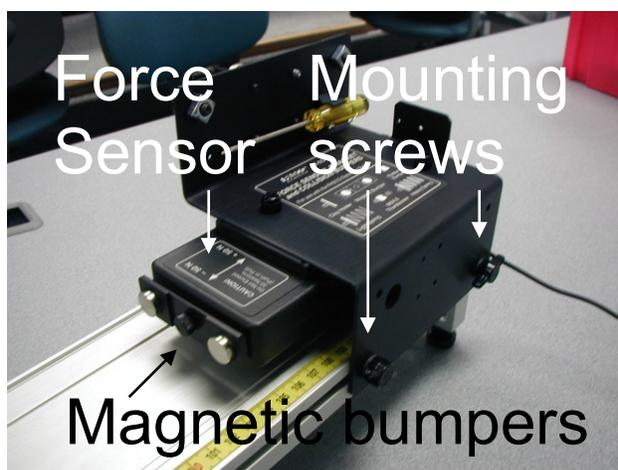
10. Hang a mass on the hanger. Using the known mass, you can calculate what the force is that is exerted on the force sensor. Enter this force in the “Standard Value” box and click the “Set Current Value to Standard Value” button. Repeat this procedure with a different weight and then press finish. The sensor should now be calibrated.
