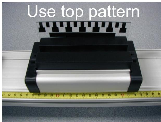
window will open that will allow you to change the “Flag Spacing.” Note that the spacing is measured in meters. Enter the correct value for the spacing of the opaque bands on your picket fence and click OK.
