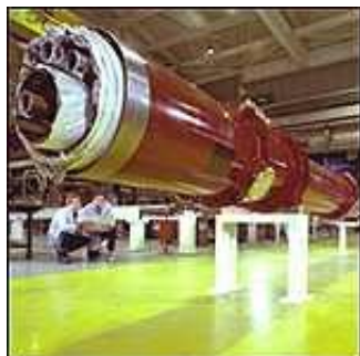
Huge magnets are needed to accelerate the particles
